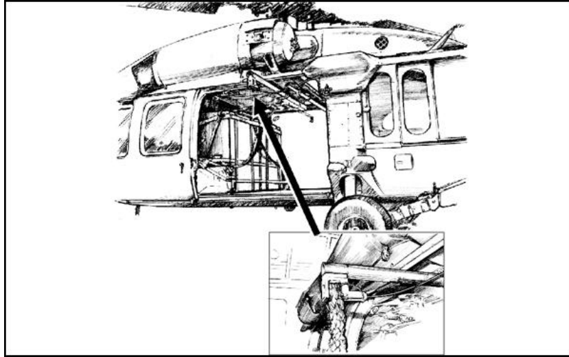
Figure 5-2. Bar assembly correctly mounted to aircraft.
